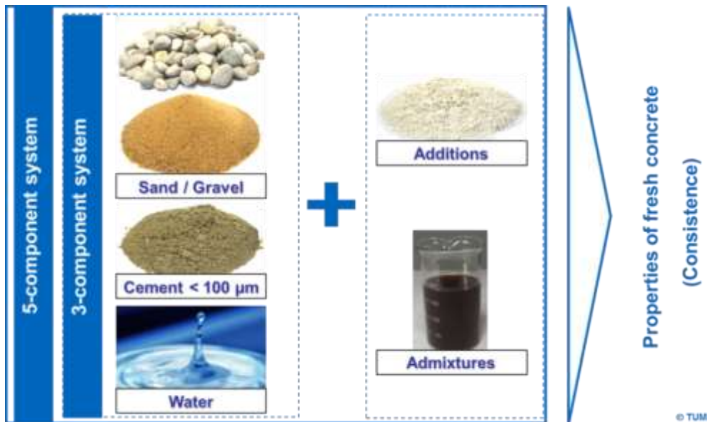
Figure 26. Modern five-component substitutes the old three-component concrete technology
