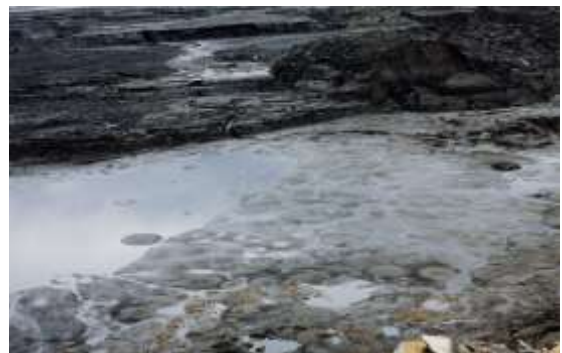
Figure 27. Evidence of tailings liquefaction
