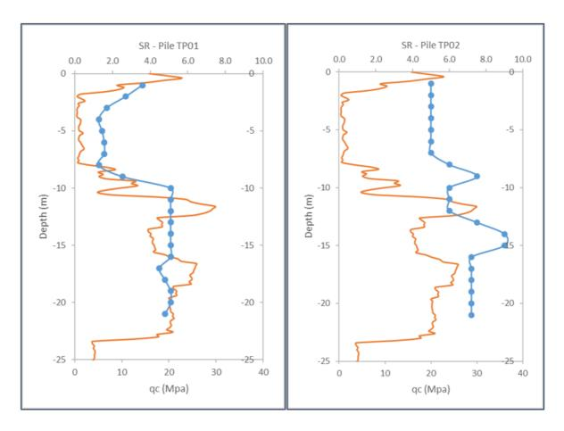
Figure 9. Antwerp jobsite – SR measured for TP1 and TP2
