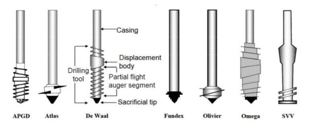
Figure 11. Drilled Displacement Piles – Current Practice and Design (Prasenjit Basu, Monica Prezzi and Dipanjan Basu, 2010)
