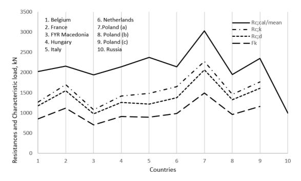
Figure 2a. Example 2 – Bored pile (T. Orr, 2016) – Resistances and characteristics loads
