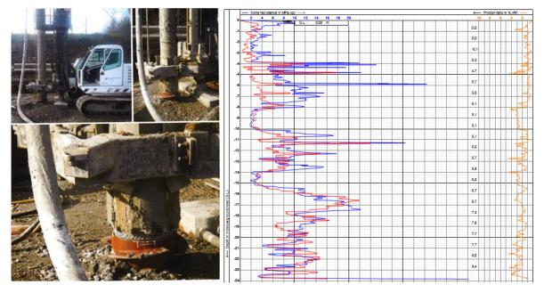
Figure 13. Haren test site - Illustration of the execution of a DA pile with grout injection (left) and results of the CPTE performed in the axis of the test pile
