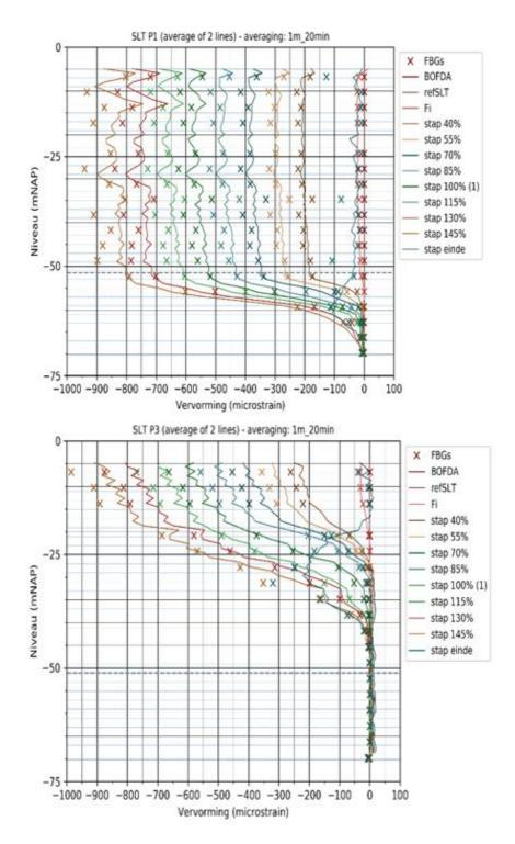
Figure 24. Results of the deformation measurements in 2 different micropile systems during a compressive load test
