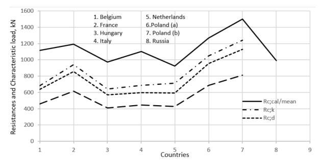
Figure 2b. Example 2 – Screw pile (T. Orr, 2016) – Resistances and characteristics loads
