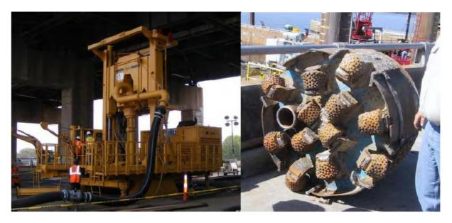
Figure 25. Reverse Circulation Drilling – limited headroom and full face drilling tool (Brown, 2012)
