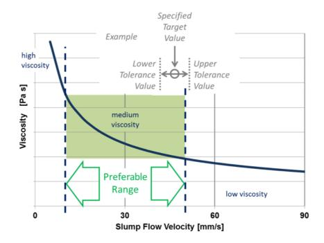
*Figure 28. Slump Flow Velocity Curve related to viscosity showing the recommended range of medium viscosity for tremie concrete*
