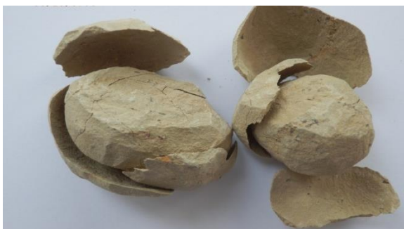
Figure 9. An example of degradation caused on marl sample by suction
