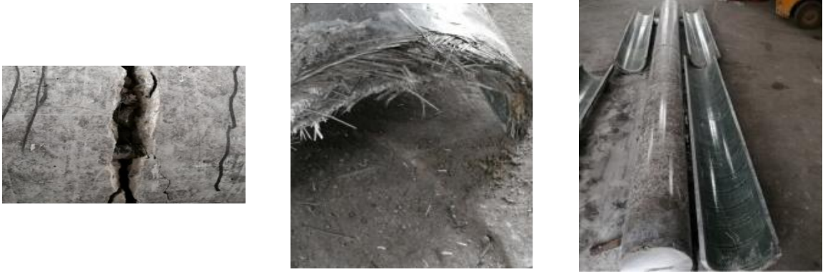
(c) Failure of the BFRP tube in the mid-span
