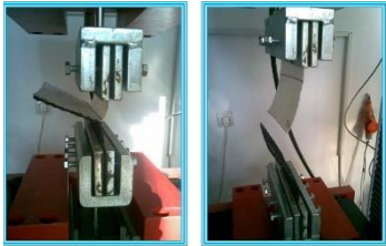
Figure 5. Example 3 – peel test on the drainage geocomposite (Batali et al, 2014)
