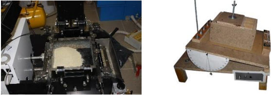
Figure 4. Example 3 – shear tests at interface (Batali et al, 2014)
