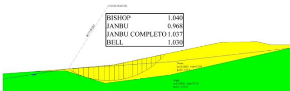
Figure 11. Case study – old landfill – LEM stability analyses static conditions, characteristic values F_s = 0.97
