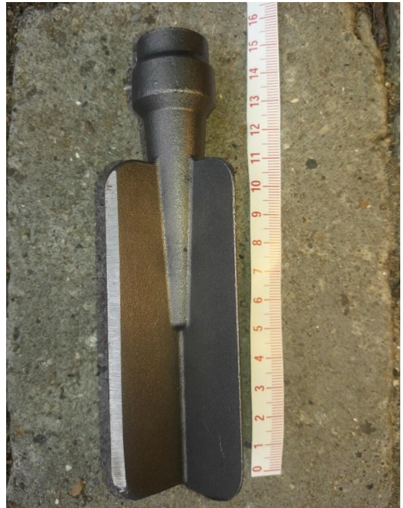
Figure 3.1. The Danish "deep vane" with sharpened edges, rounded corners and a friction reducer on top of the vane shaft.
