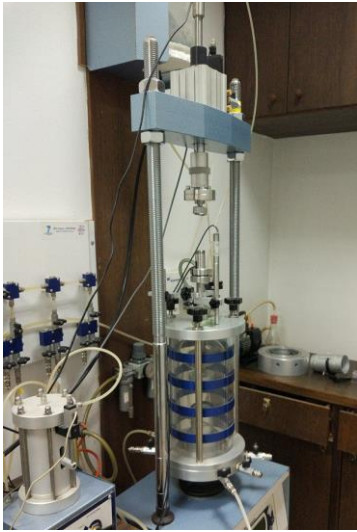
Figure 5. Dynamic triaxial apparatus
