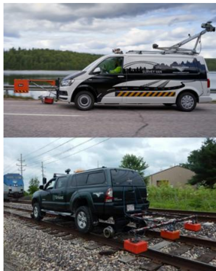
Figure 1. Above: Road Doctor Survey Van (RDSV) with 2 GHz air coupled antenna and 400 MHz ground coupled antenna in front of the vehicle. Laser scanner with IMU and GPS is located on the roof behind the vehicle. Below: HyRail vehicle equipped with three 400 MHz ground coupled antennas.
