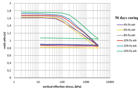
Figure 2. Void ratio- axial stress relationship for various fly ash contents at a curing time of 56 days
