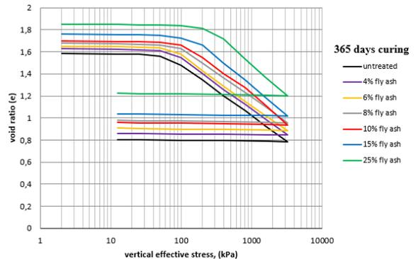
Figure 5. Void ratio- axial stress relationship for various fly ash contents at a curing time of 365 days
