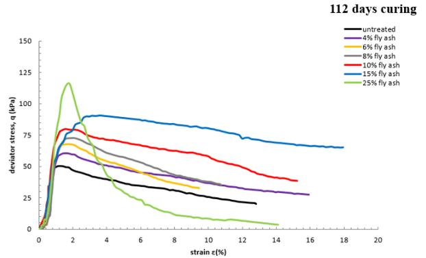
Figure 7. Effect of fly ash content on stress-strain behaviour of treated and untreated clay mixtures at a curing time of 112 days
