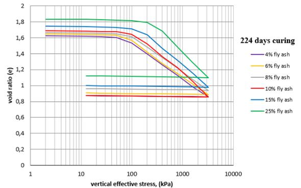
Figure 4. Void ratio- axial stress relationship for various fly ash contents at a curing time of 224 days
