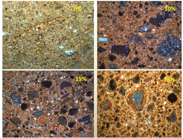
Figure 10. PLM images of fly ash treated and untreated clay mixtures
