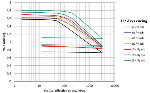
Figure 3. Void ratio- axial stress relationship for various fly ash contents at a curing time of 112 days
