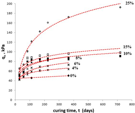
Figure 9. Effect of fly ash content on unconfined compressive strength of treated and untreated clay mixtures
