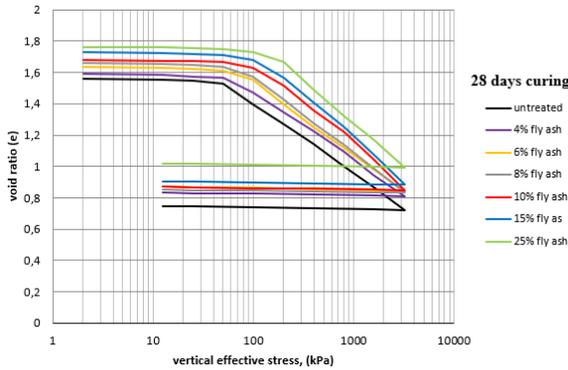
Figure 1. Void ratio- axial stress relationship for various fly ash contents at a curing time of 28 days
