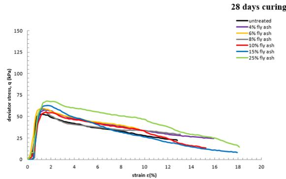
Figure 6. Effect of fly ash content on stress-strain behaviour of treated and untreated clay mixtures at a curing time of 28 days
