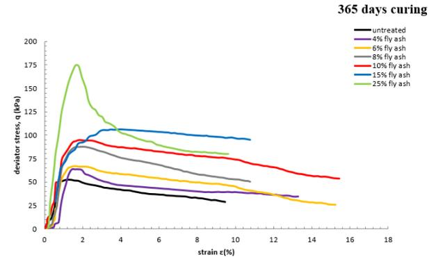
Figure 8. Effect of fly ash content on stress-strain behaviour of treated and untreated clay mixtures at a curing time of 365 days
