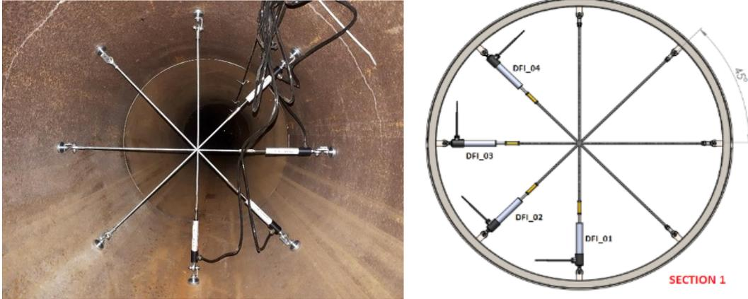
Figure 3 - Position of numbered sensors inside a sensor-equipped section of the micro-tunnel and corresponding photo.
