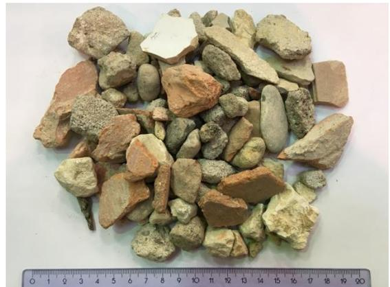
Figure 1. Sample of recycled aggregate used in this study (ruler in centimetres)
