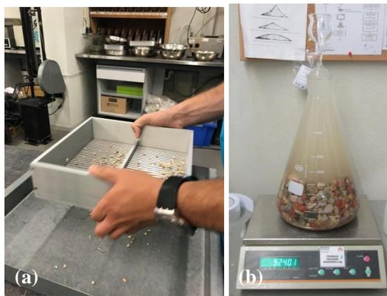
Figure 3. Characterization of the recycled aggregate: a) determination of flakiness index; b) determination of particle density and water absorption
