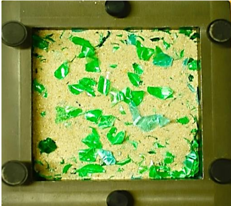
Figure 5. Soil-Plastic Composite placed in the 100 mm by 100 mm direct shear box
