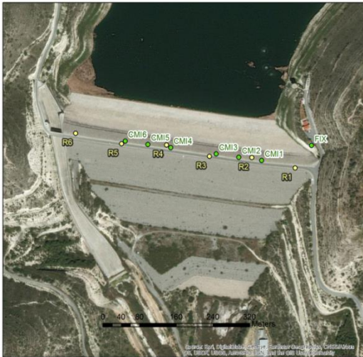
Figure 2. Instrumentation on the dam crest
