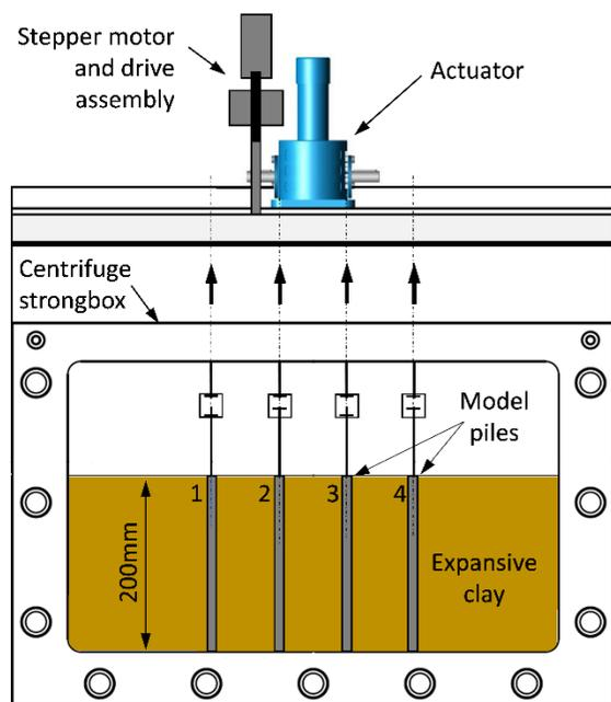
Figure 1. Model setup and instrumentation
