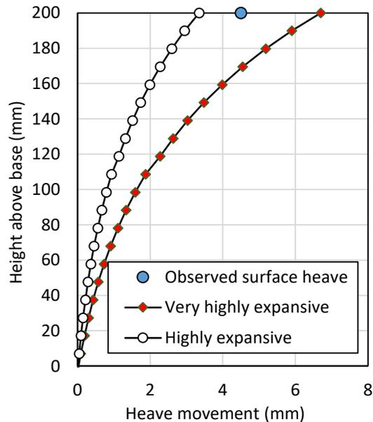
Figure 7. Observed surface heave compared against heave profiles by Van der Merwe (1964)
