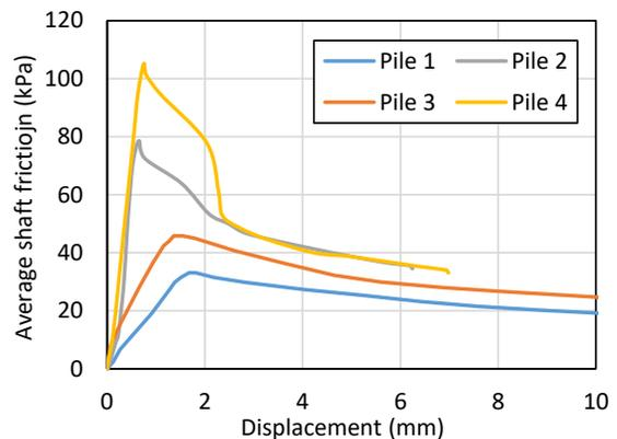
Figure 9. Pile shaft friction
