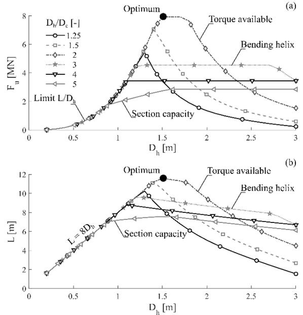
Figure 5 Uplift capacity  $F_u$  and installation length  $L$  of a screw pile embedded in dense sand as a function of the helix diameter  $D_h$  and  $D_h/D_c$  ratio, assuming a maximum installation torque equal to  $5\text{MNmm}$
