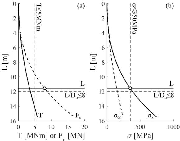
Figure 6 Determination of the maximum embedment and uplift capacity of a screw pile embedded in dense sand for a given geometry ( $D_h=1.5\text{m}$ ,  $D_h/D_c = 2$ ,  $t_h = 0.1\text{m}$ ,  $t_c = 0.075\text{m}$ ) and maximum installation torque ( $T_{max} = 5\text{MNm}$ )
