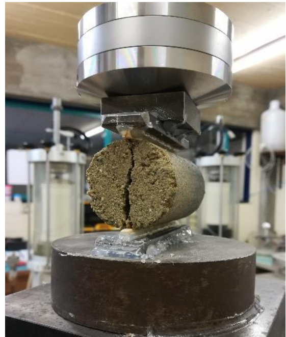
Figure 2. Split tensile strength test
