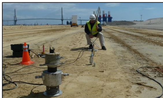
Figure 2. Performance of SASW test near borehole S1
