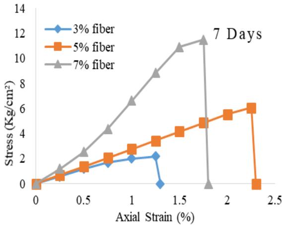
Figure 1. Stress-strain curves with different cement content after curing for 7 days
