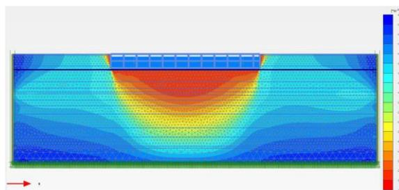
Figure 7. Settlements due to dewatering
