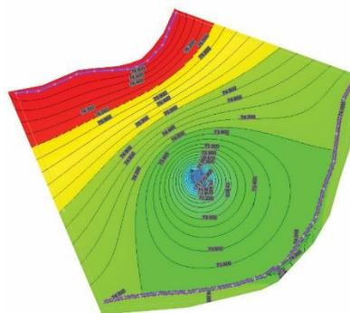
Figure 6. Hydro-dynamic spectrum with the influence of dewatering
