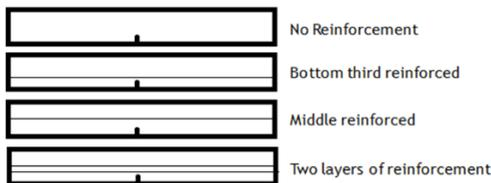
Figure 1. Location of Geosynthetic Reinforcements
