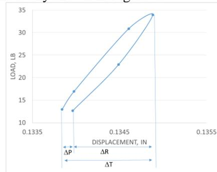
Figure 5. Permanent Deformation for each Cycle in a typical Fatigue Testing (FUN-1)
