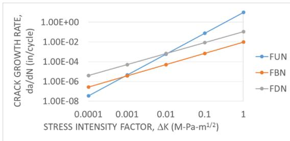
Figure 7: Paris' Law for Unreinforced, Bottom-Third Reinforced and Double Reinforced Beams
