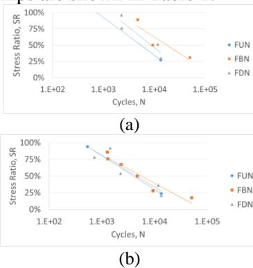
Figure 4: Stress Ratio vs. Number of Cycles to Failure for Fatigue Tests on Notched Beams (a) Approach 1 and (b) Approach 2
