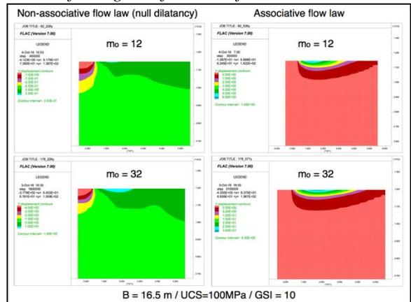
Figure 7. The variation of the vertical displacements under the footing as a function of  $m_0$ .
