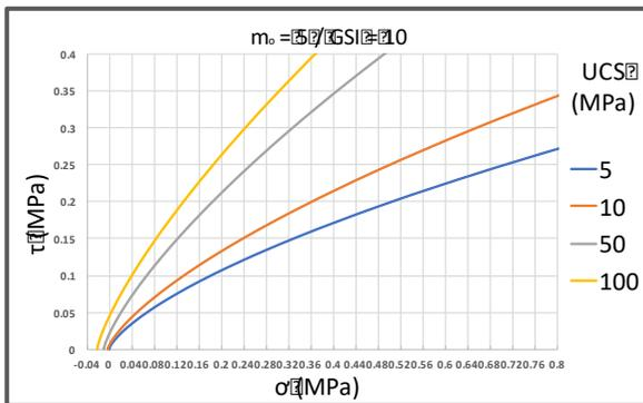
Figure 3. Representation of the Hoek and Brown failure envelope.
