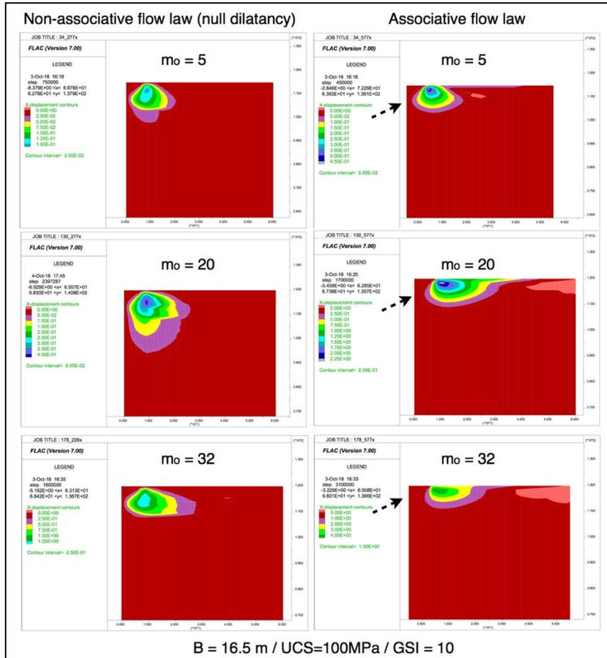
Figure 6. The variation of the horizontal displacements under the footing as a function of  $m_0$ .
