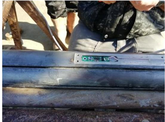
Figure 2: Electronic board inserted in the slotted tube
