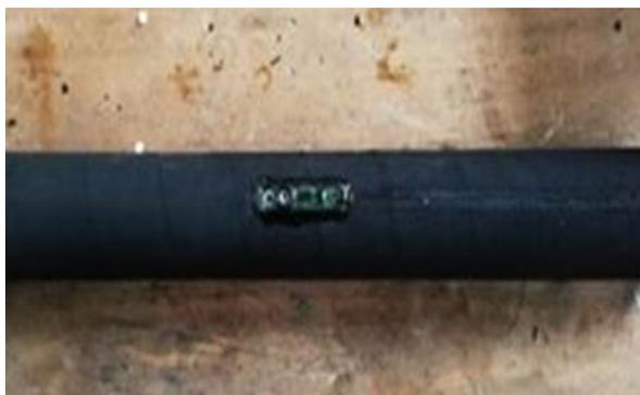
Figure 4: Sensor integrated in the flexible rubber
