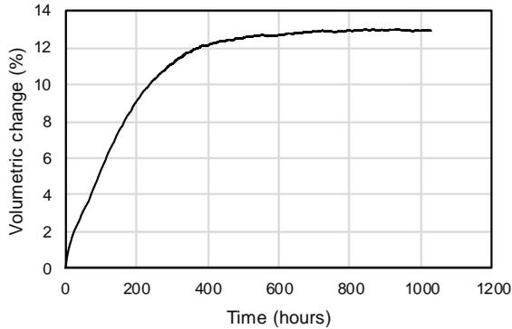
Figure 4. Swell under 50 kPa (sand-bentonite mixture)
