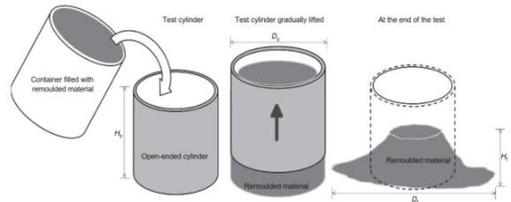
Figure 3: Description of slump test procedure ; (Thakur2014)
