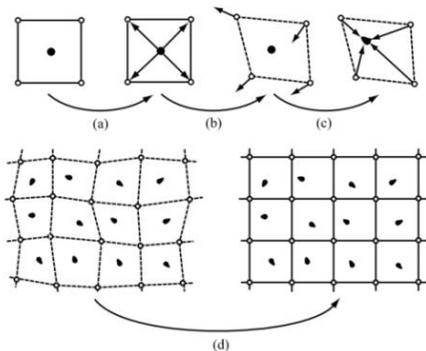
Figure 2: Schematic illustration of the MPM algorithm (Zhang, 2016).
