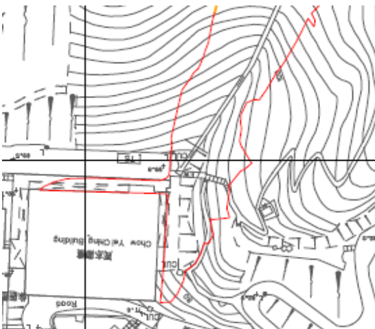
Figure 4. Graphical output (plan view) of the LS-DYNA simulation at 70.0s (top) compared to the actual debris trail (extracted from LSR3/2009) (bottom).
