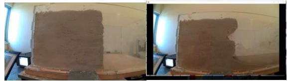
Figure 17. Snapshots of the semi-submerged, vertical slope failure (Test No. 8)
