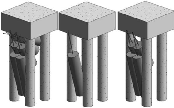
Figure 2. Indicative grouting stages at foundation locations as planned, TaM 1, 4 and 8 from left to right.
