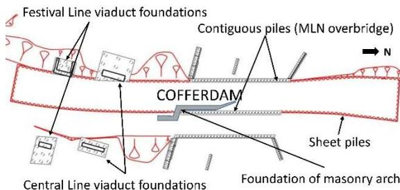
Figure 1. Cofferdam and site constraints
