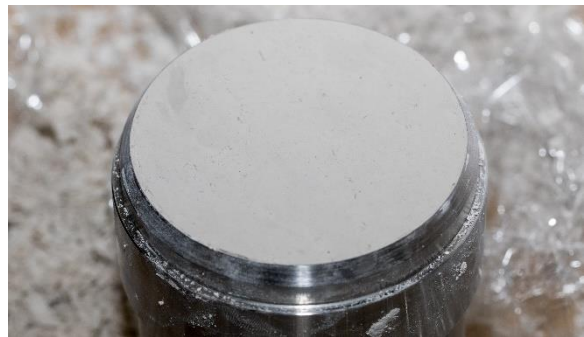
Figure 6 pressing-out in drilled core sample. Chalk sample prepared in the oedometer ring ready for testing.
