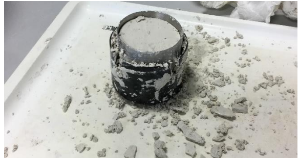
Figure 5 pressing-out in drilled core sample. The \text{\O}70\text{mm} ring were pressed into the core sample, which reduced the number and size of cracks significantly.
