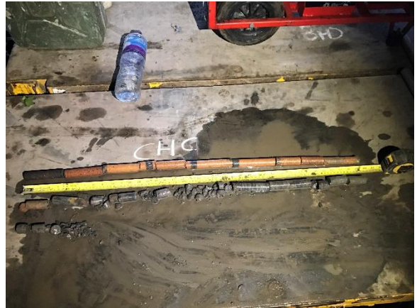
Figure 8 – Example of core recovery from Lonlas Tunnel
