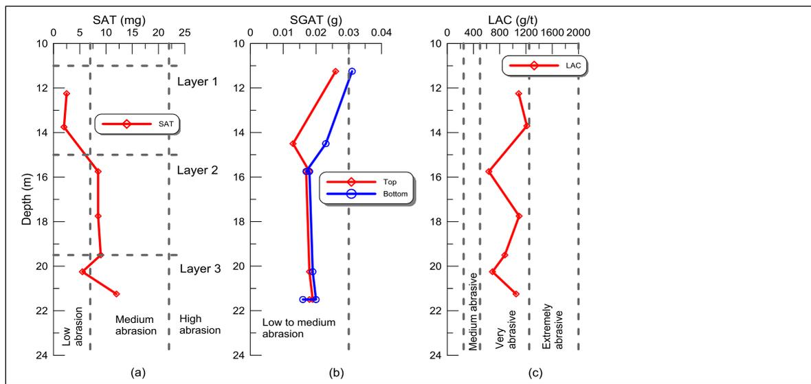
Figure 6. Results of (a) SAT, (b) SGAT and (c) LCPC abrasion testing
