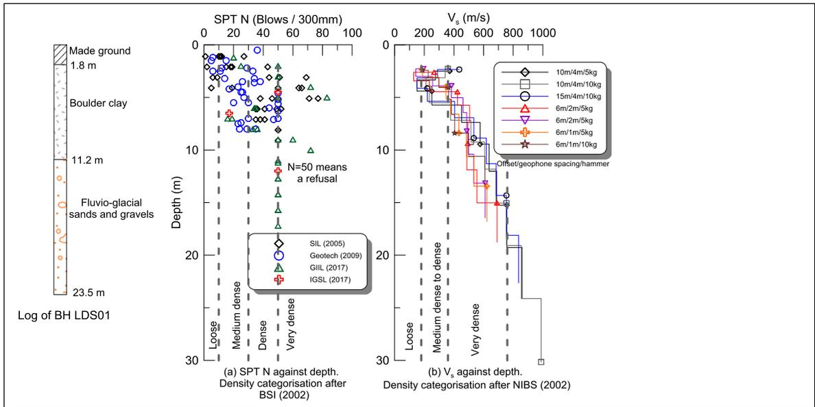
Figure 5 Standard penetration test (SPT) and MASW surface wave test results
