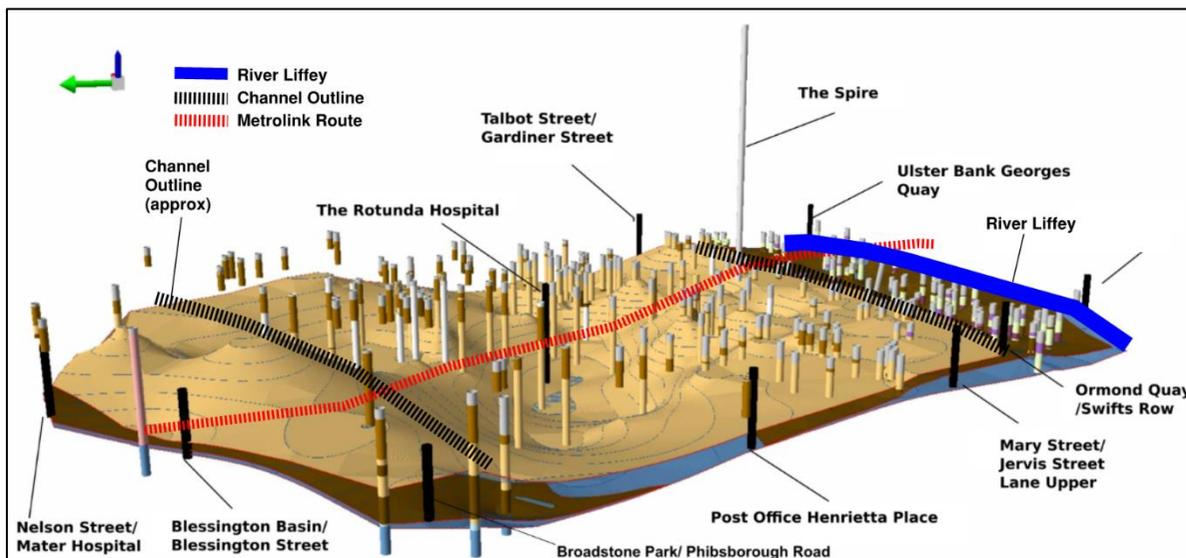
Figure 4. 3D image of ground model showing distribution of fluvio-glacial materials (yellow) and glacial till on the flanks (brown)
