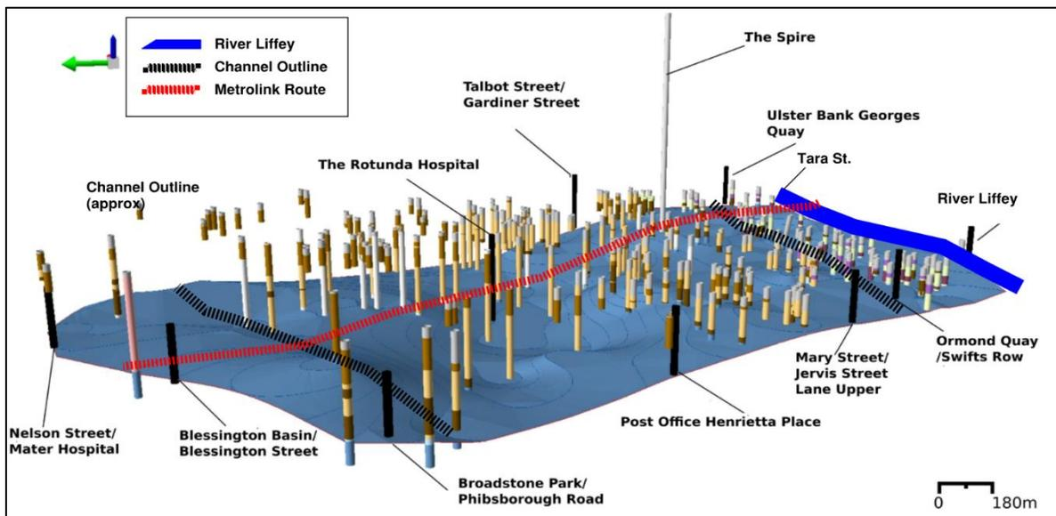
Figure 3. 3D image of ground model showing bedrock profile (blue)
