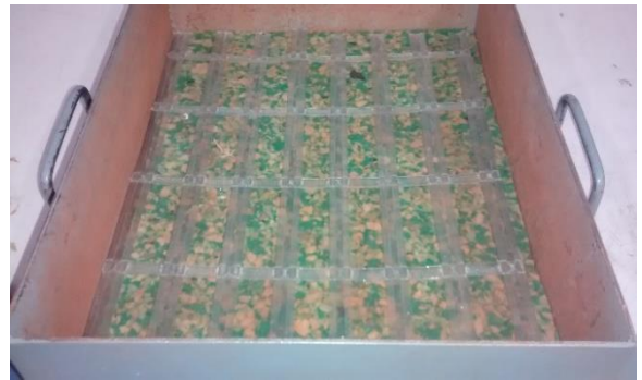
Figure 6. View of the geogrid placed on top of the sponge during specimen preparation
