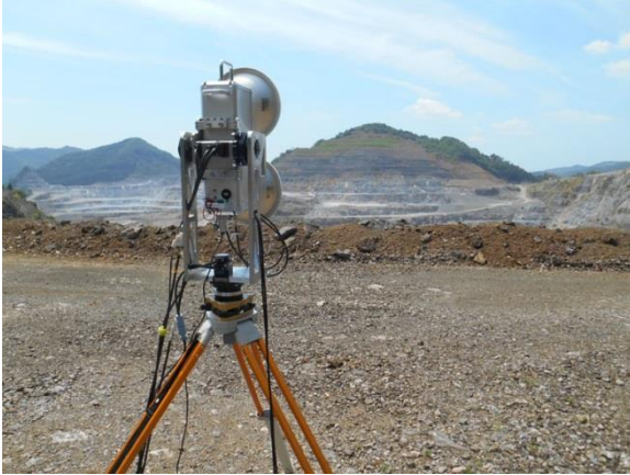
Figure 1. Appearance of ground-based millimeter wave radar.
