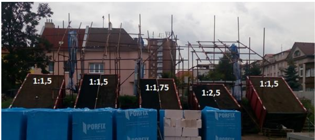
Figure 1: Photo of the testing setup with 5 areas (containers) with indication of the applied slopes
