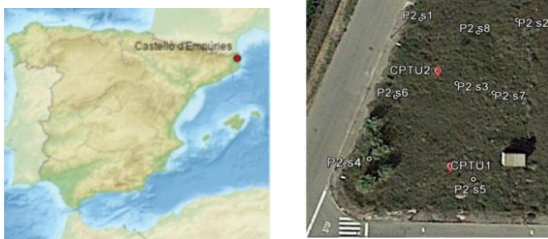
Figure 2. Test site location (dot) and implantation of piezocone tests (CPTU) and Panda tests (P2Si)
