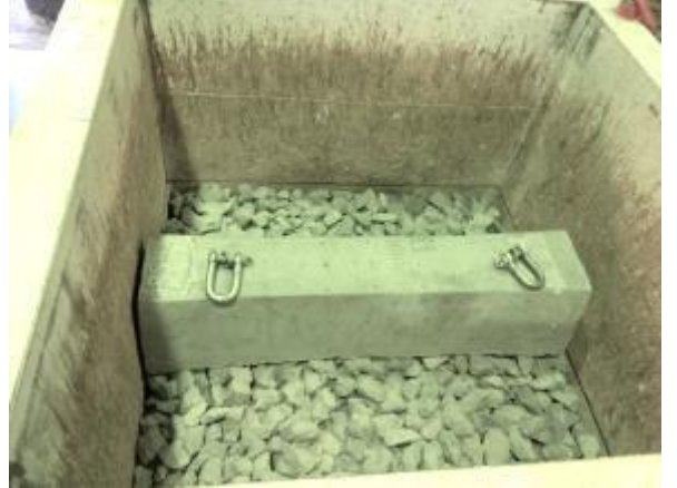
Figure 5 Placement of the sleeper on the ballast layer at shear plane
