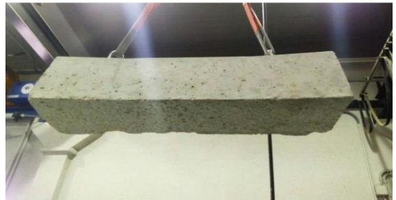
Figure 6 Inspection of bottom sleeper surface
