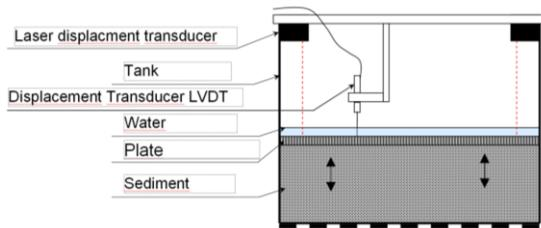
Figure 1. Scheme of the sedimentation tank
