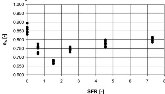
Figure 2. Initial void ratio of tested samples
