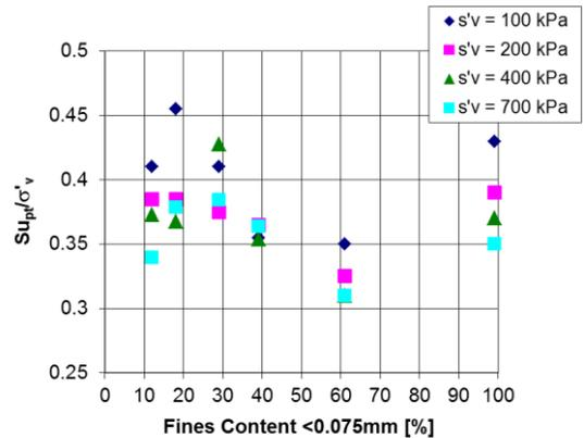
Figure 13. Influence of fine fraction content on normalized undrained shear strength .
