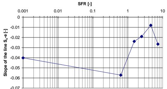
Figure 12. Effect of the SFR index on the slope of the line describing the relationship between undrained shear strength in and the void ratio.
