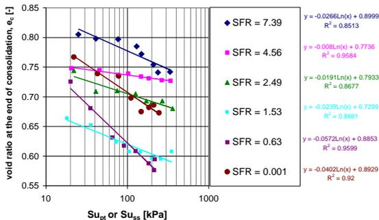
Figure 11 Relation between undrained shear strength and void ratio at the end of consolidation stage.
