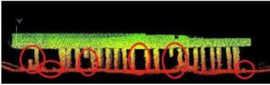
Figure 6. Reconstruction of the river bed profile from the bathymetric survey (from Hera Report, 2018)
