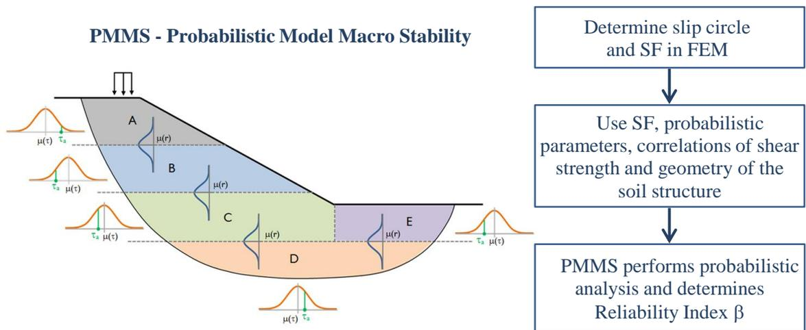
Figure 1 Main principles in the PMMS - Probabilistic Model Macro Stability
