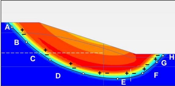
Figure 4 Geometry with failure mechanism and shear band elements, denoted with a letter. The + and - signs are correlation indicators
