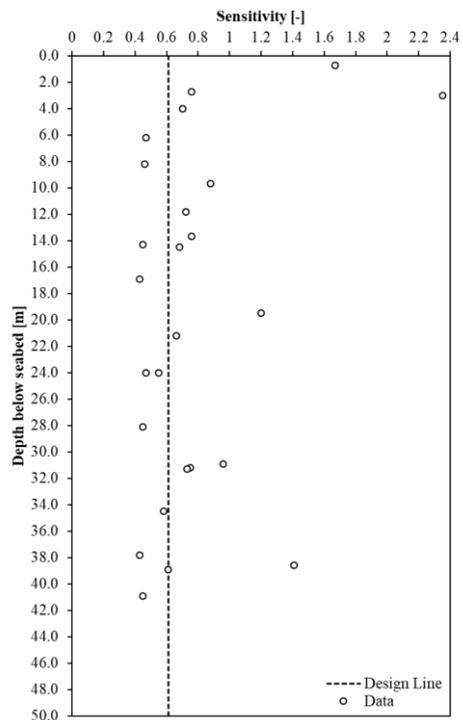
Figure 2. Clay sensitivity distribution with depth
