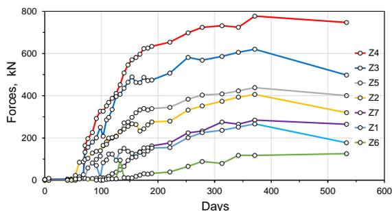
Figure 10. Tensile forces in the monitored micropiles
