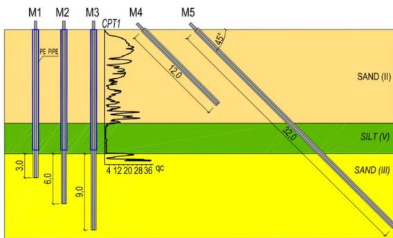
Figure 9. Scheme of tested micropiles
