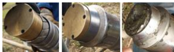
Figure 8. GP-S operation: (a) key components; (b) device assembled; (c) activated core catcher.
