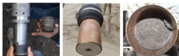
Figure 7. D&M operation: (a) key components; (b) device assembled; (c) liner after sampling.
